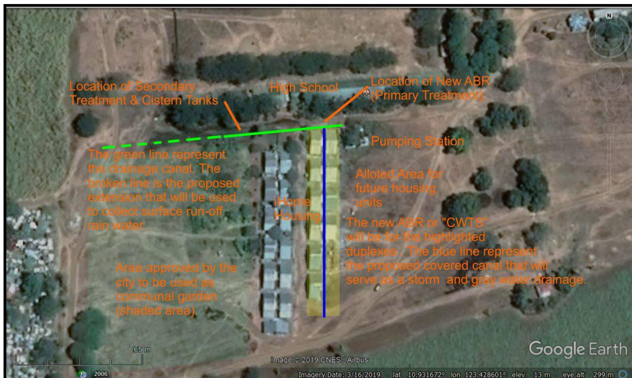
Picture No. 1: Site Development Plan of iHome Housing featuring wastewater treatment and re-cycling.
