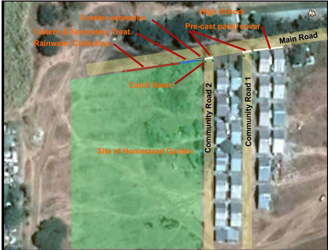
Picture No. 3: Additional 5 meters of drainage canal and pre-cast panels to cover parts of canal.
